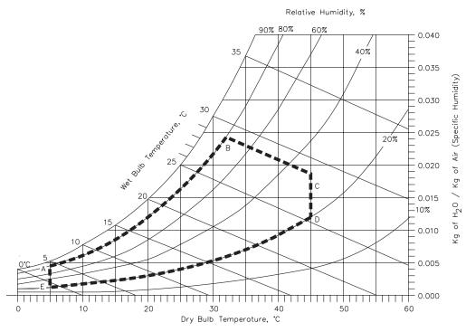
Figure 7-3 Internal model: Operating temperature and humidity ranges
